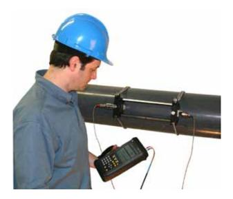
To hold clamp-on transducers in contact with the pipe, a variety of clamping fixtures are available to accommodate different pipe and transducer sizes. These fixtures use a variety of attachment methods including chain, metal strap, Velcro® strap and magnetic clamps.
