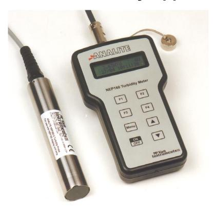
The ANALITE NEP160 is a truly portable turbidity meter. Readings are taken by simply inserting the probe into the steam or media to get an immediate result truly representative of the turbidity level at that point and time. It allows for easy and fast multiple readings at a site to ascertain the real turbidity profile of a stream or water body.
