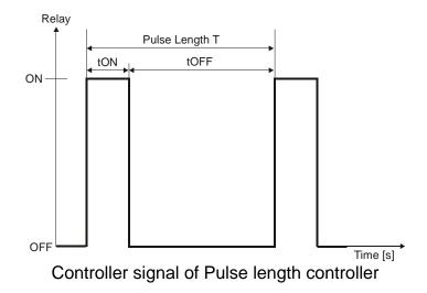
The output relay of the pulse length controller is clock-timed. The switching period T remains constant. Depending on the divergence from the limit value, the switch-on time  $t_{\text{ON}}$  is increased or decreased in accordance with the proportional range Xp.
