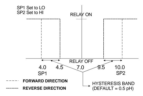
The controller relay activates when the set-point is reached. In the reverse direction, it does not de-activate when the value reaches the set-point. Instead, it continues to be active till the value reaches the amount set by the Hysteresis band.
