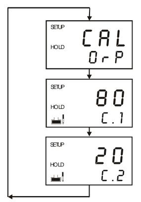
To calibrate the controller for ORP %:
