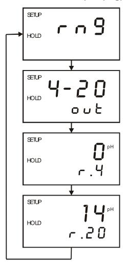
This sub-function lets you set the controller current output range of this unit.
