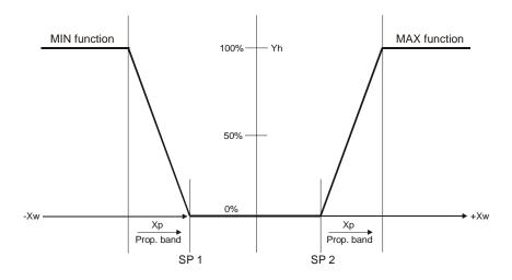
Control characteristic of P-Controller as proportional controller
