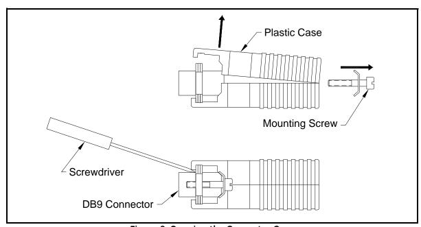
Figure 9: Opening the Converter Case
