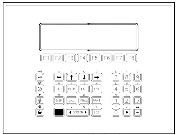
Figure 1: The Model DF868 Keypad
