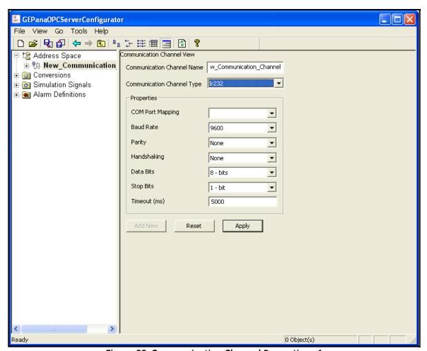
Figure 52: Communication Channel Properties - 1
