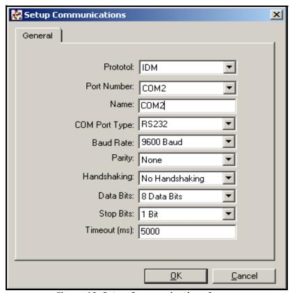
Figure 19: Setup Communications Screen
