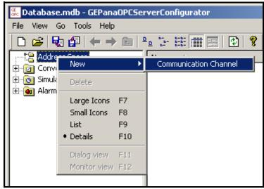
Figure 51: New Communication Channel
