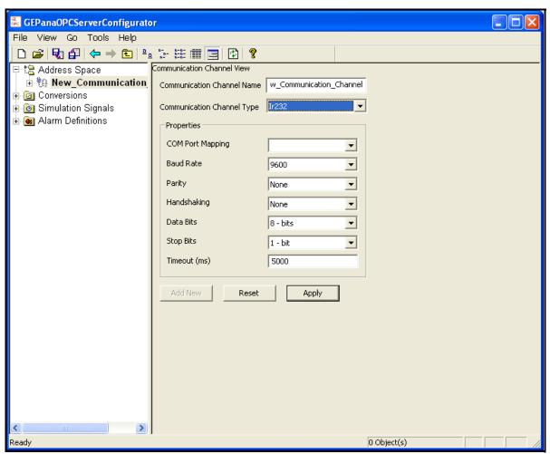
Figure 52: Communication Channel Properties - 1
