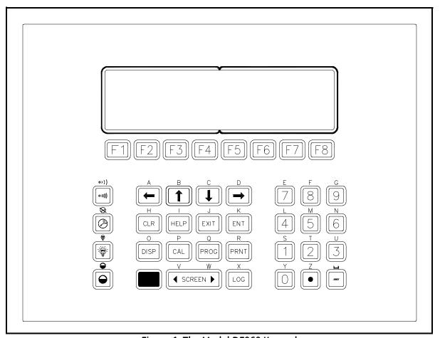
Figure 1: The Model DF868 Keypad
