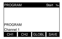
Press the  $[\bullet]$  and  $[\varnothing]$  keys and one of the function keys [F1]-[F4] to select the desired submenu. From this screen, press [EXIT] to return to measurement mode.
