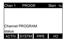
Press the  $[\bullet]$  and  $[\varnothing]$  keys and a function key [F1]-[F4] to select the desired submenu. From this screen, press [EXIT] to return to the initial *User Program* screen shown on page 1-8.
