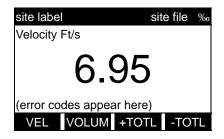
The default power up screen is already in BIG mode. If a different display mode is active, access the *Display Menu* by pressing the [DISP] key.
