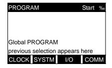
Press the  $[\bullet]$  and  $[\varnothing]$  keys and a function key [F1]-[F4] to select the desired submenu. From this screen, press [EXIT] to return to the initial *User Program* screen shown on page 1-8.
