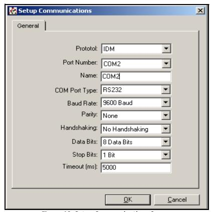
Figure 19: Setup Communications Screen
