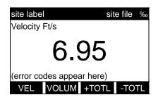
Use the [F1]-[F4], [ $\blacklozenge$ ] and [ $\varnothing$ ] keys to select the desired display parameter option. Refer to Table 27 on page 56 for a complete description of the available options.
