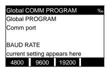
To change the baud rate, press the  $[\varnothing]$  key until the desired baud rate appears on the option bar, and then press the appropriate [Fx] function key.
