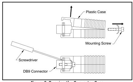
Figure 9: Opening the Converter Case
