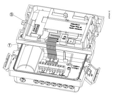
Figure 7-1 S - Verification sealing (protective seal); T - Test
