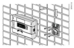
Figure 4-1 Wall mounting of the device
