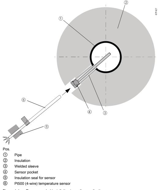
Figure 4-4 Recommended installation in cooling applications
