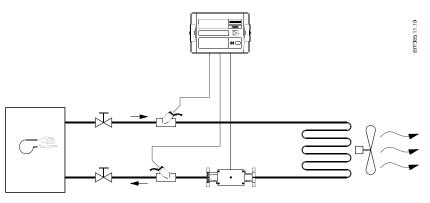
Figure A-1 District heating application with the flowmeter installed in the cold pipe
