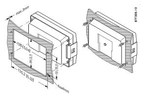
Figure 4-2 Panel mounting of the device
