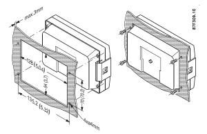
Figure 10-2 Panel mounting, dimensions in mm (in)
