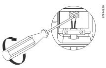
5. After installing main power cable, install protection cover using the two screws in order to avoid contact between voltage-carrying parts and cable-pull-relief, see figure below.
