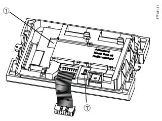
Figure 7-3 ① - Test output; T - Verification sealing / HW key
