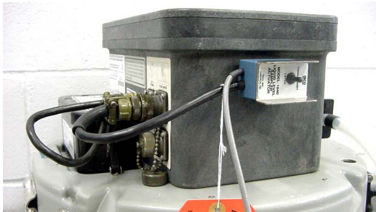
Figure 2-1 1640 Liquid Level Actuator Installed on a Sampler
