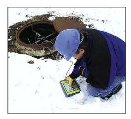
The Field Wizard can interrogate a stack containing up to four 2100 Series area velocity and ultrasonic flow modules. It can download and store more than 14 days\* of data from as many as 20 individual 2100 Series flow modules. In addition, the Field Wizard allows you to adjust level settings on the area velocity and ultrasonic flow modules.
