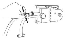
Figure 2-6 Attaching the vinyl suction line with a tube coupler
