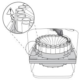
Figure 4-1 Sliding the 24-bottle rack out
