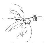
Figure 2-7 Releasing a tube coupler clamp
