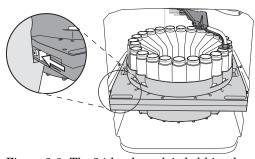
Figure 2-3 The 24-bottle rack is held in place by a latch on the left side
