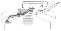
Figure 2-1 Installing the distributor arm and discharge tube
