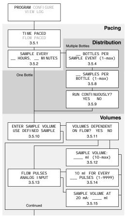
Figure 3-2 Time paced sampling program flow chart
