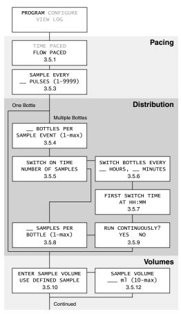
Figure 3-4 Flow paced sampling program flow chart
