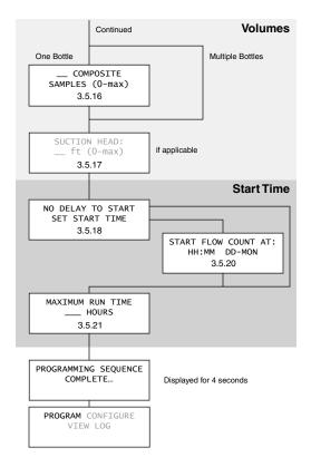
Figure 3-5 Flow paced sampling program flow chart, continued
