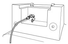
Figure 2-10 External device connection at rear of sampler
