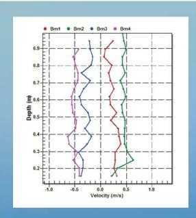
The chart above shows the individual data collected from each beam (Bm1, Bm2, Bm3, Bm4).
