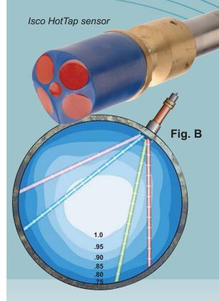
Velocity beams are range-gated, creating individual "bins" to collect data at numerous points throughout the metering section.
