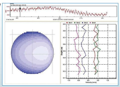
In the Flowlink screen above, a complete flow profile is clearly visible, and the accompanying chart provides velocity information at different depths.
