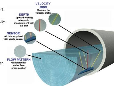
As a result, the accQpulse $^{TM}$  provides detailed velocity data in relation to sensor location at multiple points in three different directions within the flow channel. This is used to calculate a true, highly accurate flow.
