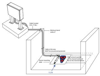
Figure 28: Installation example Rectangular channel
