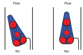
Figure 18: Sensor alignment with channel wall
