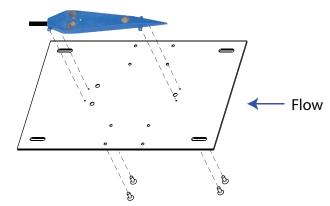
Figure 13: Sensor mounting plate
