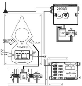
Figure 2: Wall-mounted flow meter with optional interface module
