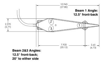
Figure 7: Shallow water sensor dimensions and beam angles
