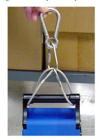
Figure 4: accQpulse suspension harness
