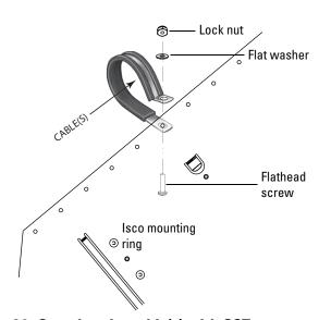
Figure 20: Securing the cable(s) with SST straps
