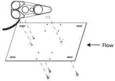
Figure 26: Attaching the sensor to a mounting plate
