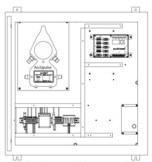
Figure 3: Console-mounted flow meter with optional interface module & heater
