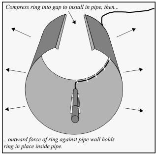
Figure 10: Spring ring compression & expansion
