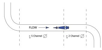
Figure 9: Sensor positioning
