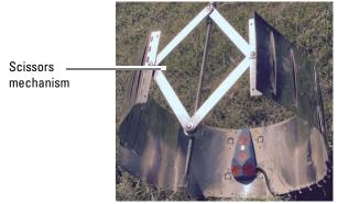
Figure 24: Ring assembled, ready for installation
