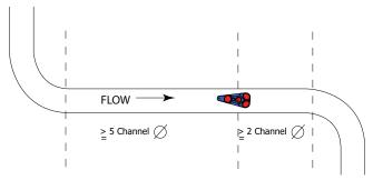
Figure 16: Sensor positioning
