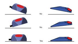
Figure 17: Mount sensor flat on channel floor
