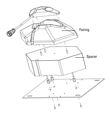
Figure 32: Sensor with fairing and fairing spacer
