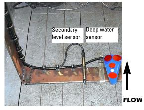
Figure 27: Rectangular frame mounting Secondary level sensor shown
