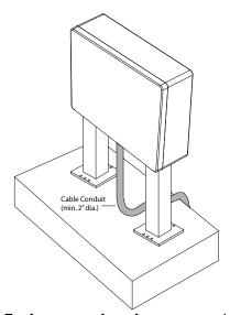
Figure 6: Environmental enclosure mounting example
