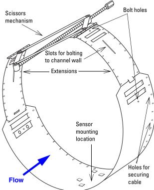
Tightening the scissors assembly expands the ring to press firmly against the pipe wall, securing the ring.
