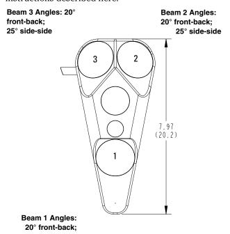
Figure 15: Sensor dimensions and beam geometry
