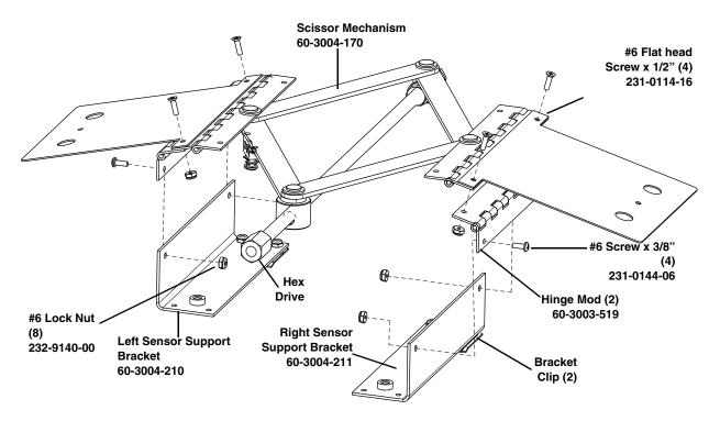
Figure 2-9 Assembling the sensor mount kit
