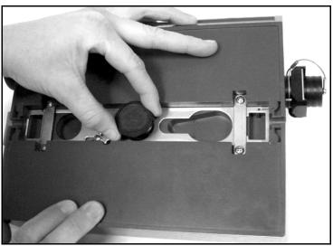
Figure 1-17 Flow Module - Unplugging the connector
