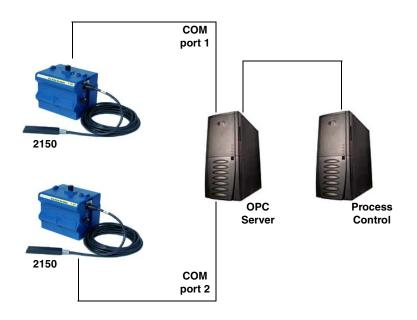
Figure 4-1 Configuration example
