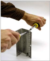
Figure 2-8 Assemble the hinges and brackets
