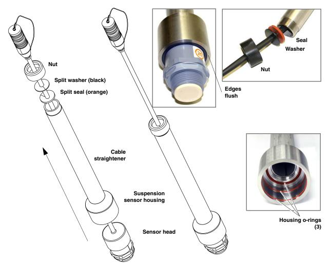
Figure 2-6 Sensor installation: Suspension
