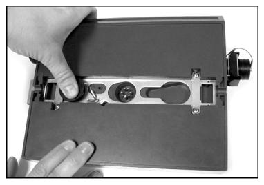
Figure 1-18 Flow Module - Pushing plug into holder
