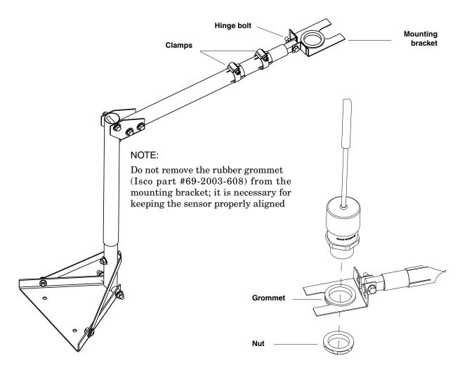
Figure 2-5 Sensor installation: Floor mounting
