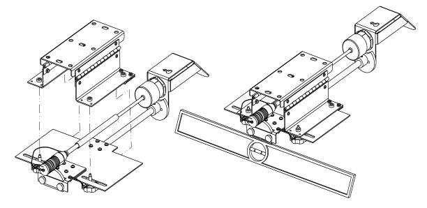
Figure 2-22 Assembling the Large In-Pipe mounting system
