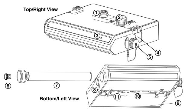
Figure 1-1 Controls, Connectors, and Indicators – 2110 Flow Module
