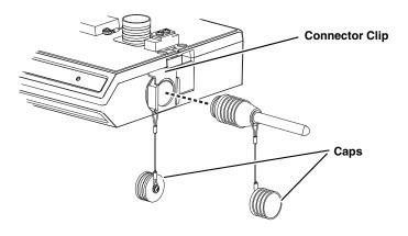
Figure 2-3 Connecting the USLS
