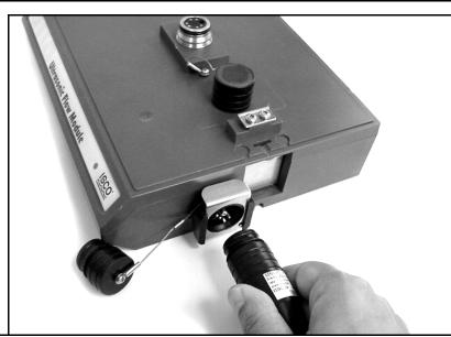
Figure 1-11 Flow Module - connecting the sensor
