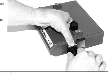
Figure 1-10 Flow Module - preparing the sensor connectors
