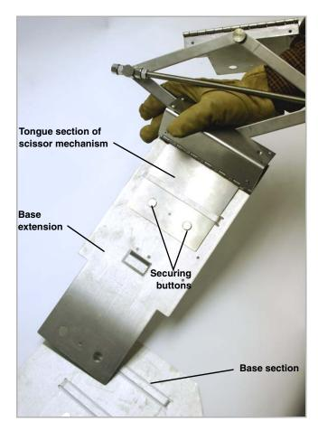
Figure 2-11 Connecting the scissor mechanism to a base extension
