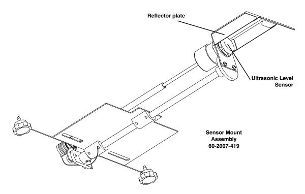
Figure 2-17 Sensor attached to the mounting assembly
