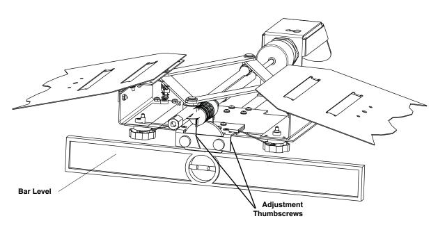
Figure 2-19 Adjusting sensor position
