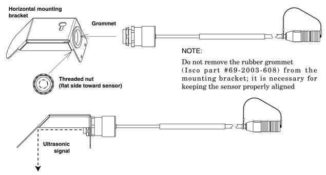
Figure 2-16 Attaching the sensor to the horizontal bracket
