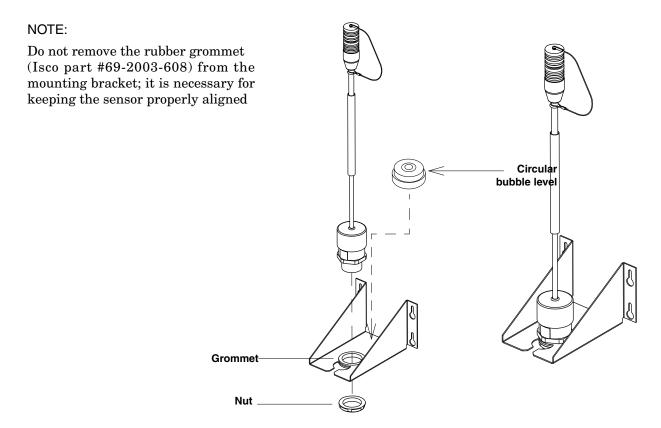
Figure 2-4 Sensor installation: Wall mounting
