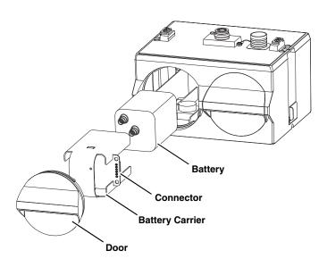
Figure 2-1 Installing a Battery
