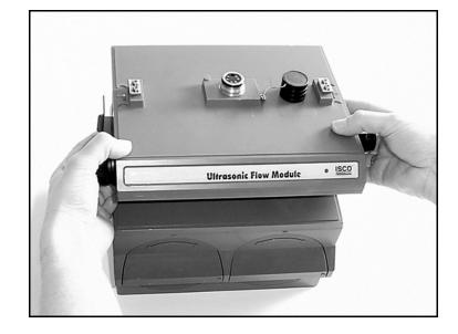
Align the modules and gently press the 2110 module down onto the 2191 module.
