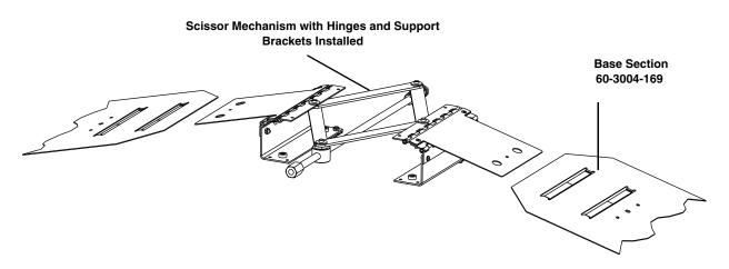
Figure 2-13 Attaching the scissor mechanism to the mounting ring
