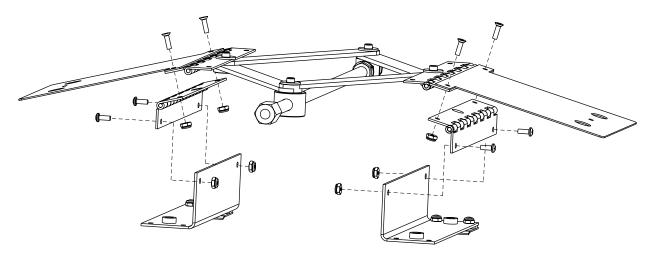
Figure 2-10 Sensor mount assembly with sensor support brackets reversed
