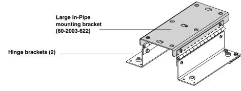
Figure 2-21 Preparing the Large In-Pipe bracket
