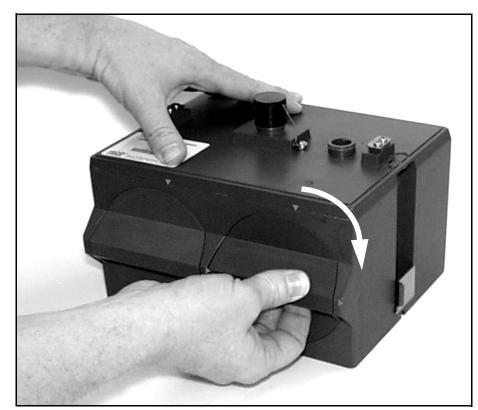
Rotate the door <sup>1</sup>/4 turn clockwise.
