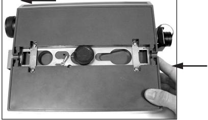
Figure 1-16 Flow Module - Unlocking the latch
