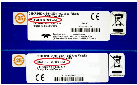
Figure 2-1 Identifying the 2150 voltage specification
