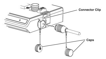
Figure 2-5 Connecting the AV Sensor
