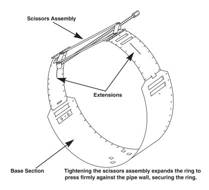
Figure 2-8 Scissors Ring adjustment
