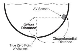
Figure 3-3 Zero Level Offset Measurement
