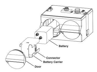
Figure 2-3 Installing a Battery
