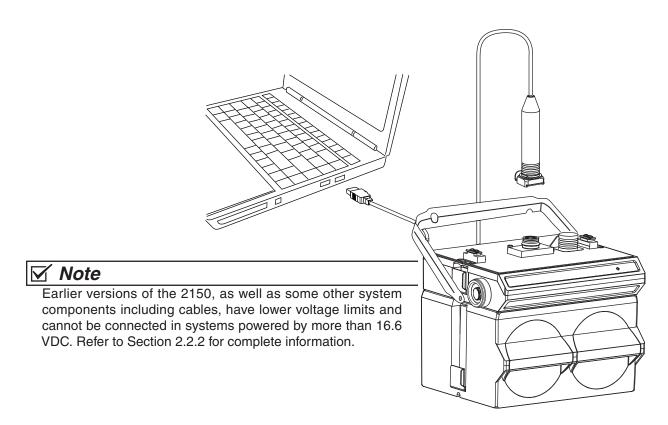
Figure 3-1 Flowlink connections
