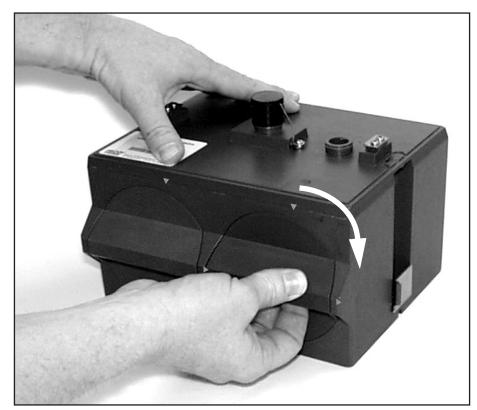
Rotate the door <sup>1</sup>/4 turn clockwise.
