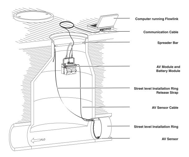
Figure 2-6 Typical Round-pipe Installation
