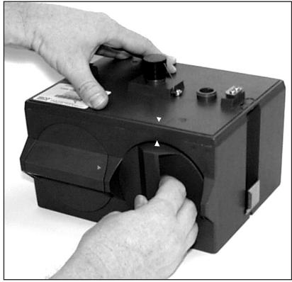
While holding the door in your right hand, align the marks and insert the door.
