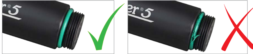
Figure 10-25 Levellogger O-ring Damage
