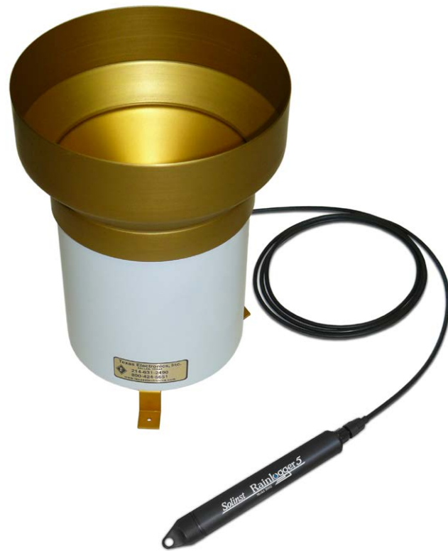
Figure 10-21 Rainlogger 5 Connected to Tipping-bucket
