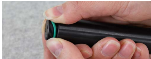
Figure 10-26 Replacing Levellogger O-rings
