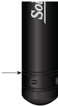
Figure 8-6 Logger Measurement Line
