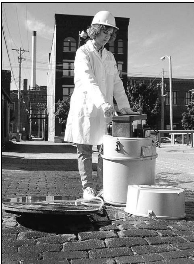
Figure 2-5 Placement of the Sampler Adjacent to Manhole
