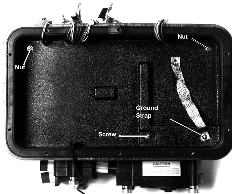
Figure 6-4 Control Box Tray Removal
