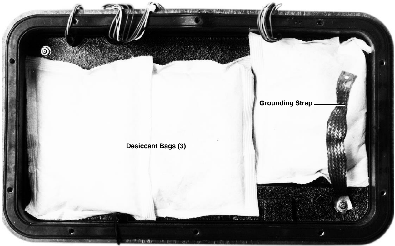
Figure 5-5 Internal Desiccant (controller lid removed)
