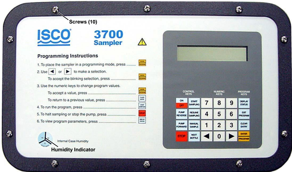
Figure 5-4 Location of 10 Screws on Control Box Lid
