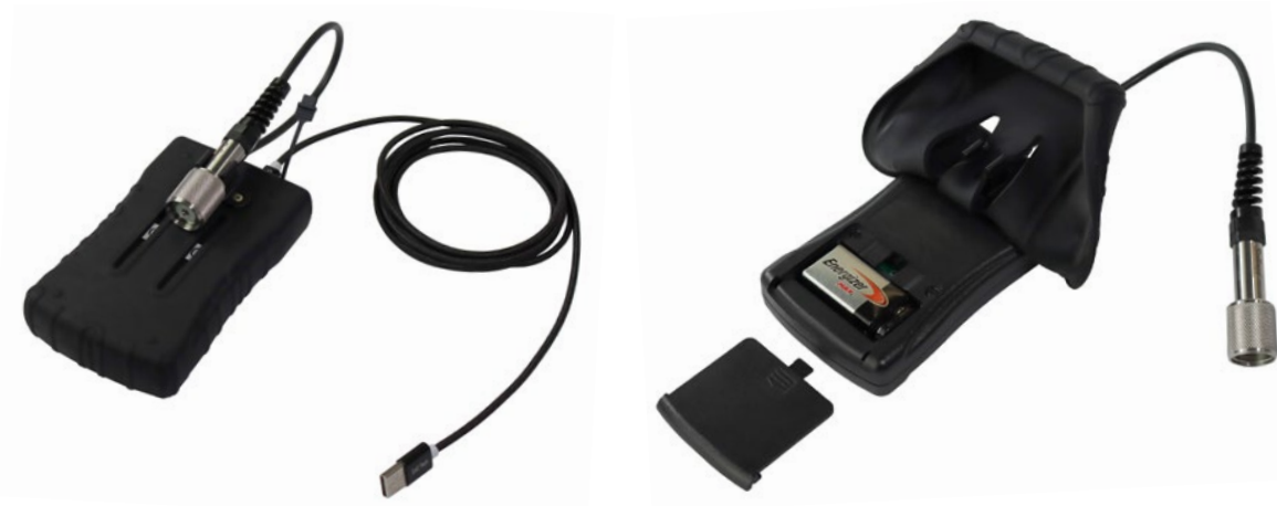
Figure 8-1 SRU Battery Installation
