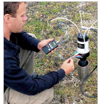
Collecting a sample from a dedicated DVP and taking pressure measurements with Model 404 Geokon Vibrating Wire Readout (above).
