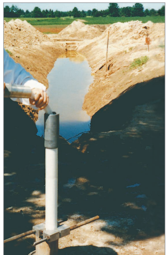
Underground oil pipeline leak assessment. Three 45 m (150 ft) installations. Two point rising head permeability tests were conducted in each interval of the Multilevel System. (See diagram showing contaminant distribution at left.)
