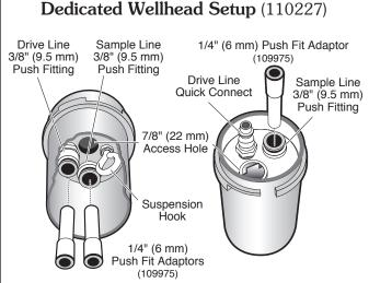
Wellheads come with three 1/4" push fit adaptors so that either 1/4" or 3/8" tubing can be used, as preferred.
