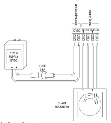
Figure 2-4 Power Supply and Analog Output Connections
