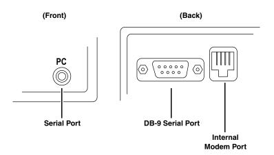
Figure 3-1 Communication Port Connectors
