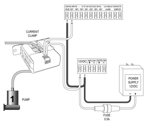
Figure 2-3 Connecting a Single Current Clamp
