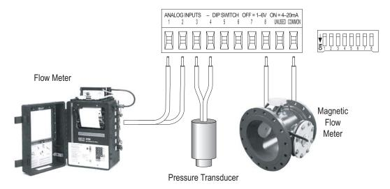
Figure 2-5 Analog Input Examples
