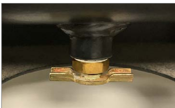
Draining valve is open
