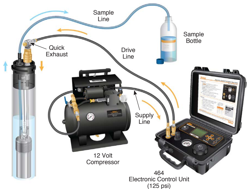
Figure 3-1 Pumping Set Up
