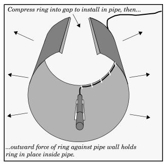
Figure 2-1 Sensor Installed on a Spring Ring
