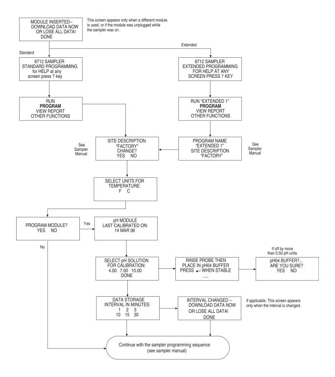
Figure 1-1 Programming the sampler to use the 701 Module
