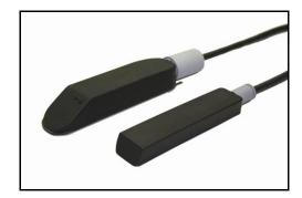
Isco offers both standard and low-profile area velocity sensors to meet you specific needs. The standard sensor (left) is most suitable in larger pipes and turbid flows with high concentrations of suspended solids and entrained air. An extended-range version of this sensor is available. See back.
