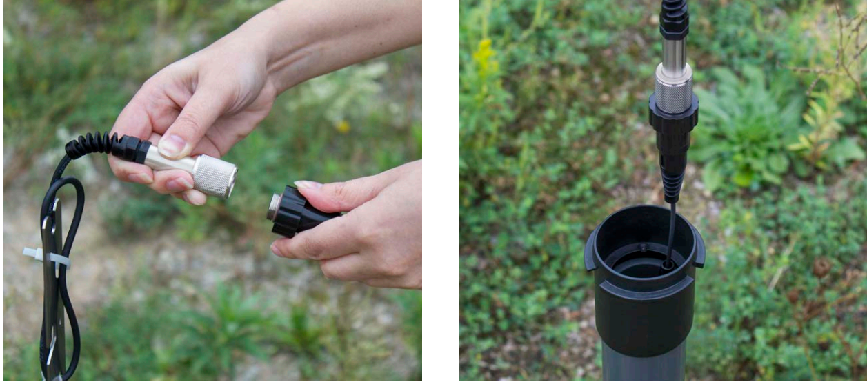
Figure 6-5 Connect the Direct Read Cable and Levellogger
