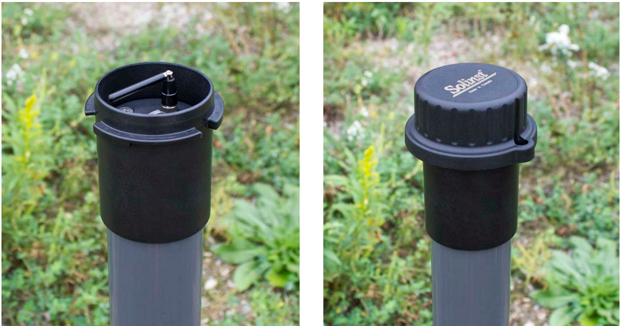
Figure 6-9 Install the Well Cap
