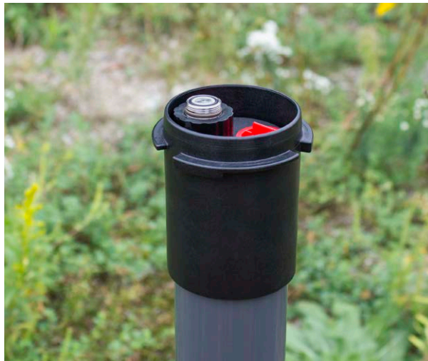
Remove Existing Levellogger Installation
