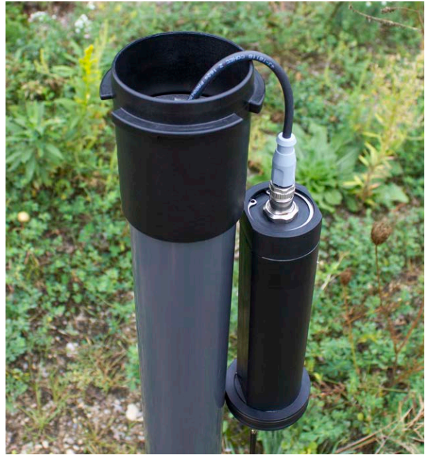
Figure 6-7 Connect the Reader Cable to the LevelSender
