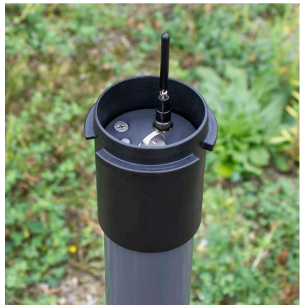
Figure 6-8 Lower the LevelSender into Position
