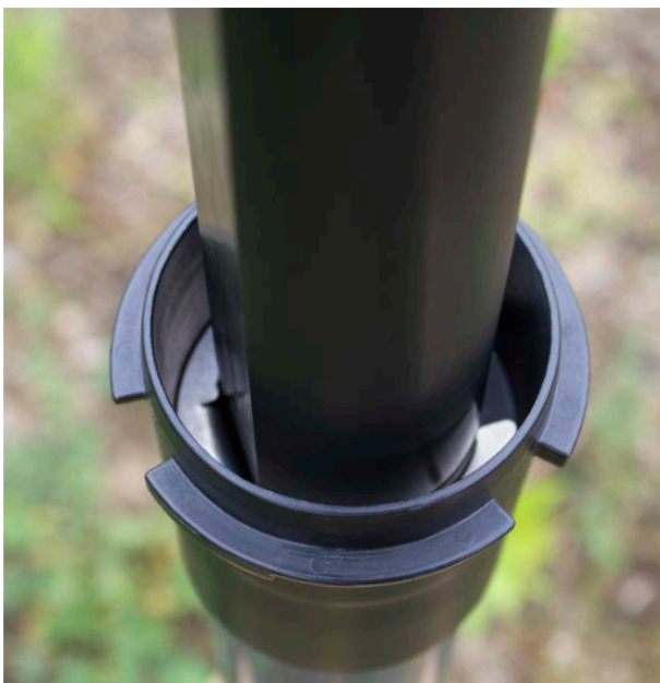
Figure 6-8 Lower the LevelSender into Position
