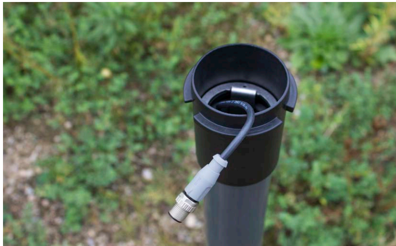
Figure 6-6 Lower the Assembly into the Well
