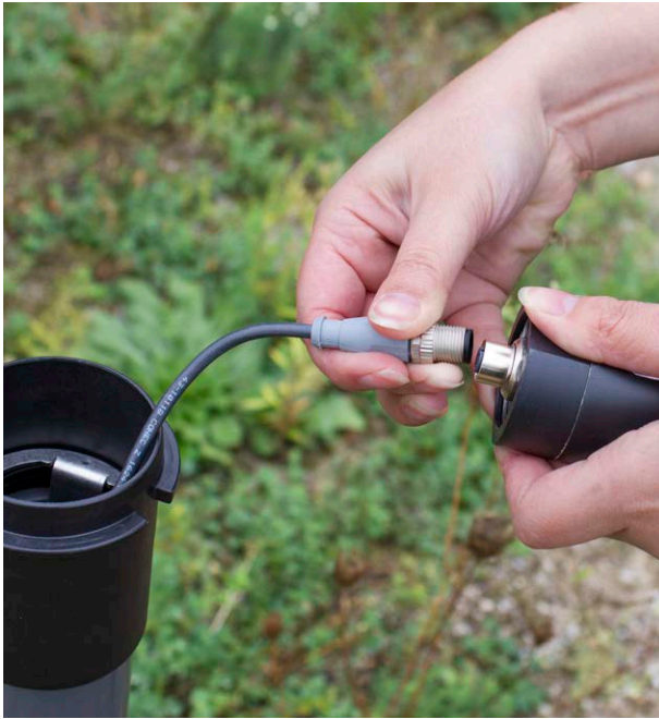
Figure 6-7 Connect the Reader Cable to the LevelSender
