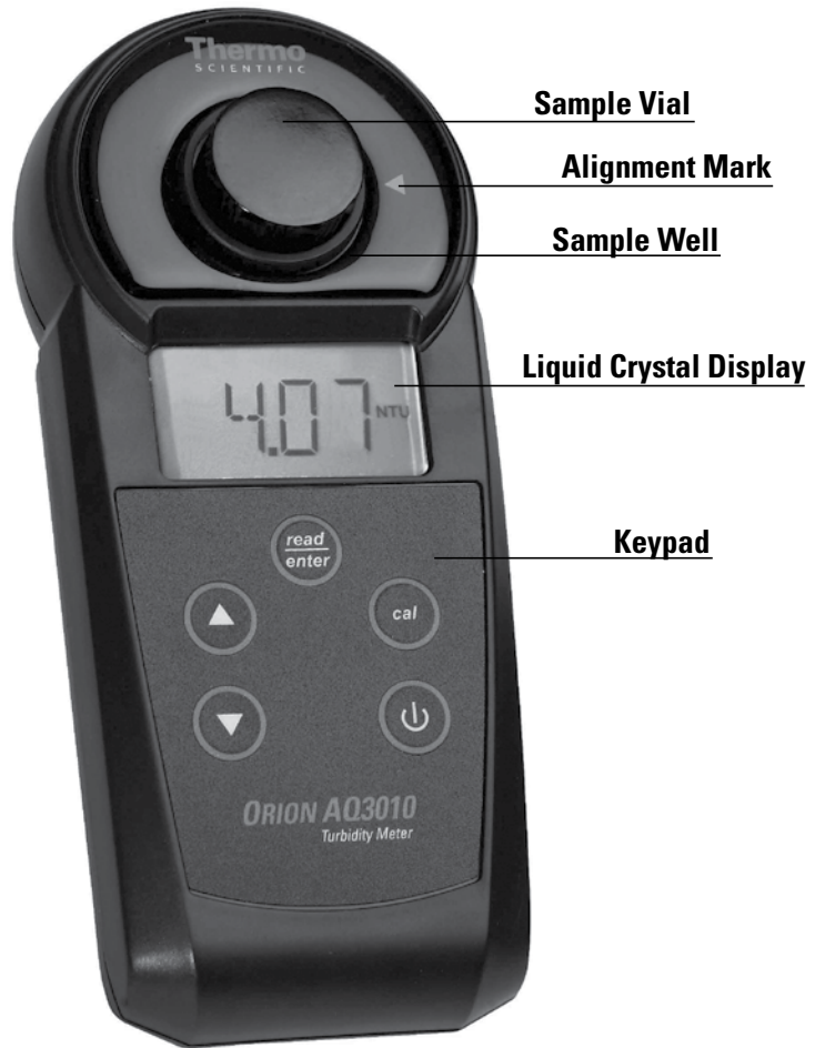
Figure 1 AQ3010 Turbidity Meter Components
