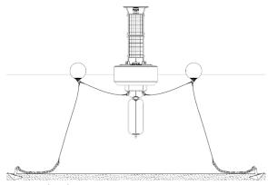
Used when monitoring sensors are deployed in the water column directly below the buoy
