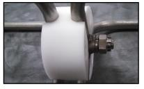
Place the end plates over the center bolt and secure with the three remaining bolts, lock washers and nuts. Tighten each securely.
