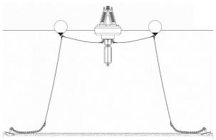
Used when monitoring sensors are deployed in the water column directly below the buoy
