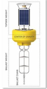
Warning: Always follow safe marine and boating practices. Heavy anchors, ballast weights and chain require careful maneuvering. Small boats with limited lifting equipment and boat clutter can be unsafe. Care must be taken during deployment to maintain a clean and safe environment.
