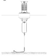
Used when sensors are attached to the instrument cage or housed in deployment pipes
