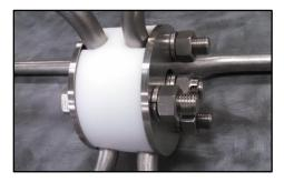
Run the cotter pin through the hole in the center bolt and bend the long leg around one of the ridges on the castle nut.
