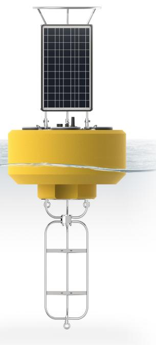
The NexSens CB-1250 Data Buoy is designed for deployment in lakes, rivers, coastal waters, harbors, estuaries and other freshwater or marine environments. The floating platform supports both topside and subsurface environmental monitoring sensors including weather stations, wave sensors, thermistor strings, multi-parameter sondes, Doppler current profilers and other monitoring instruments.
