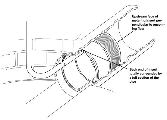
Figure 2-9 Insert Installed in Sewer Pipe
