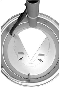
Figure 2-4 Weir Plate, Installed
