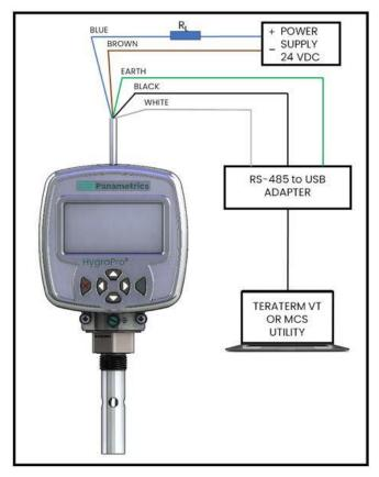
Figure 9: Standard connections with a PC
