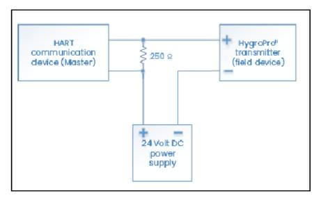
Figure 13: Point-to-point HART connection where up to 2 master devices can be used with HygroPro<sup>II</sup>
