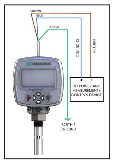
Figure 7: Standard connection to Process Controller via Analog Output
