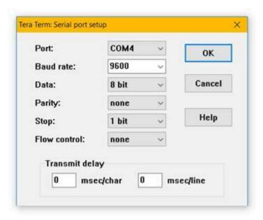
Figure 23: Serial Port Setup
