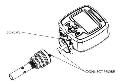
Figure 18: Removing the Hygro<sup>II</sup> RTE probe from the transmitter
