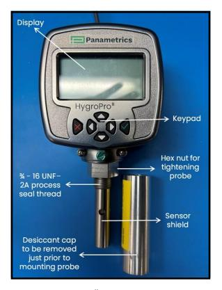
Figure 3: Key HygroPro<sup>II</sup> parts relevant to installation
