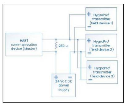
Figure 14: Multi-drop HART connection showing multiple HygroPro<sup>II</sup> transmitters, each with a unique address, connected to a single HART master
