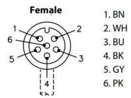
Figure 21: Pin Out for 6 Pin Female M8 Connector
