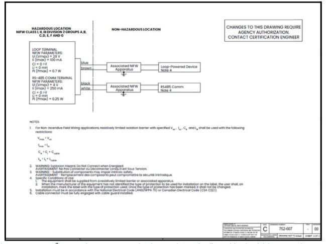
Figure 11: HygroPro<sup>II</sup> Installation Control Drawing for Non-incendive field wiring in Division 2 locations (refer to 752-607)
