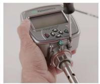
Figure 19: Reinstalling the Hygro<sup>ll</sup> RTE probe into the dismounted transmitter
