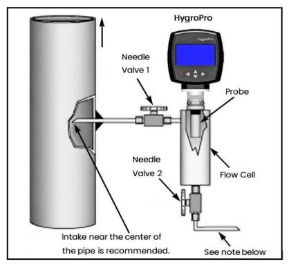
Figure 2: A Typical Sample System
