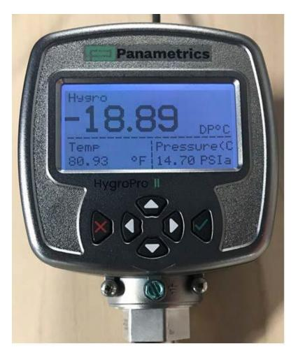
Figure 15: HygroPro<sup>II</sup> Display and Keypad
