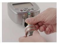
Figure 17: Step-by-step removal of the Hygro<sup>ll</sup> RTE probe from the transmitter
