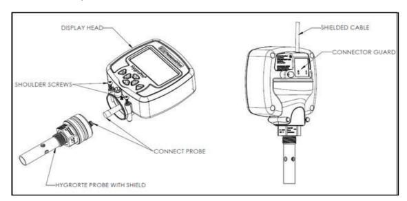
Figure 1: Major components of the HygroPro<sup>II</sup> – the display head and HygroRTE probe assembly
