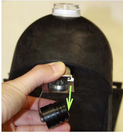
Figure 2-8 Preparing the LaserFlow connector receptacle
