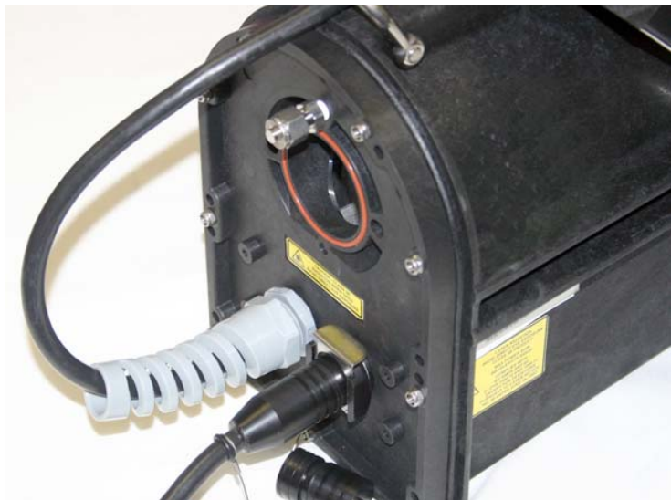
Figure 5-6 Connecting the 350 AV sensor to the LaserFlow
