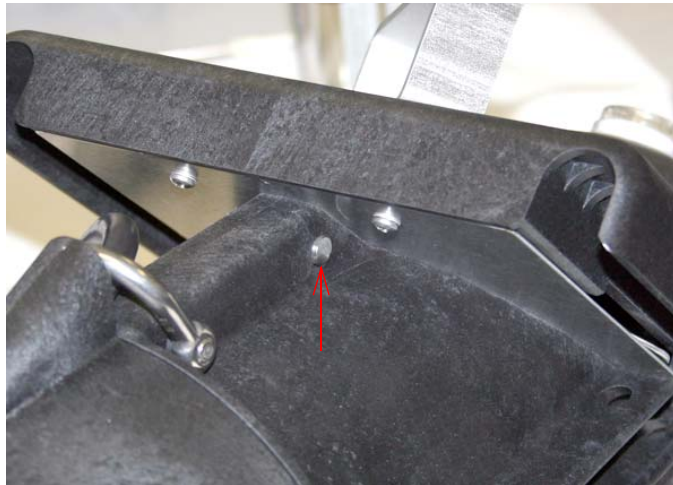
Figure 5-2 Location and orientation of cross-pins for mounting block installation
