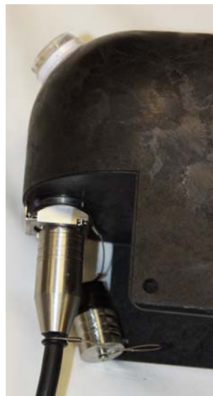
Figure 2-9 Secure caps and connect 310 ultrasonic plug to LaserFlow
