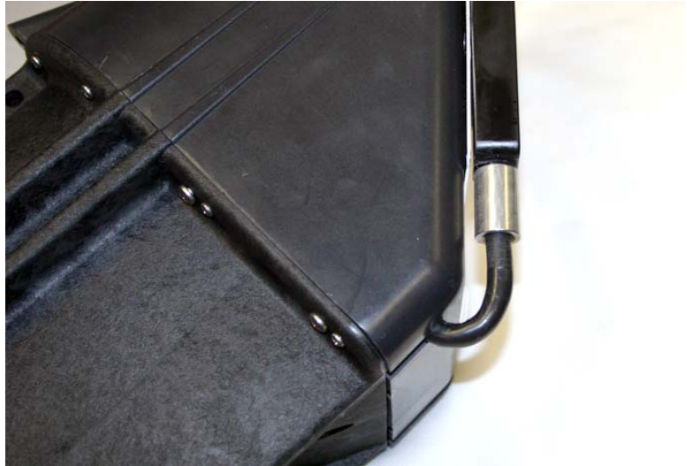
Figure 5-7 Reassembling the LaserFlow w/ AV sensor installed
