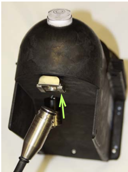
Figure 2-9 Secure caps and connect 310 ultrasonic plug to LaserFlow
