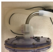
Figure 5-5 Connecting the vacuum / pressure line
