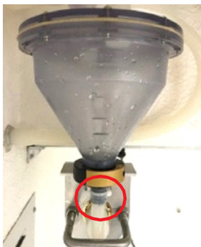
Figure 5-3 Location of the chamber discharge fitting
