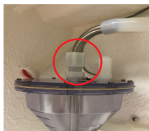
Figure 5-4 Center fitting with the compression nut
