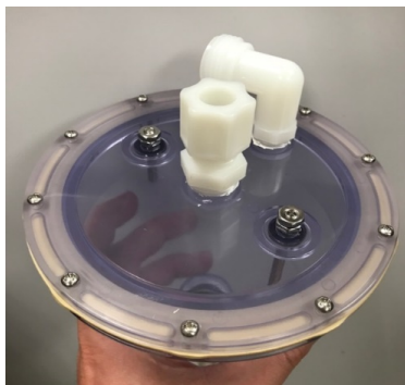
Figure 5-2 Sample Chamber Inlets (Graduation marks on this side)
