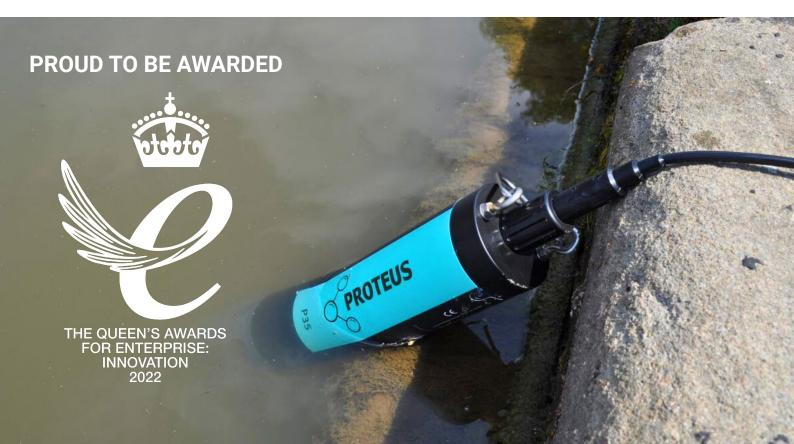
**Self cleaning:** As it is essential that optical sensors have a cleaning mechanism, the Proteus is also supplied with an integral wiper which cleans all of the Proteus' sensors before every measurement cycle.
