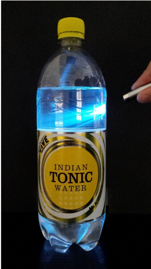
Figure 1: Example of quinine sulphate molecules in tonic water emitting blue light when exposed to high energy (UV) light.
