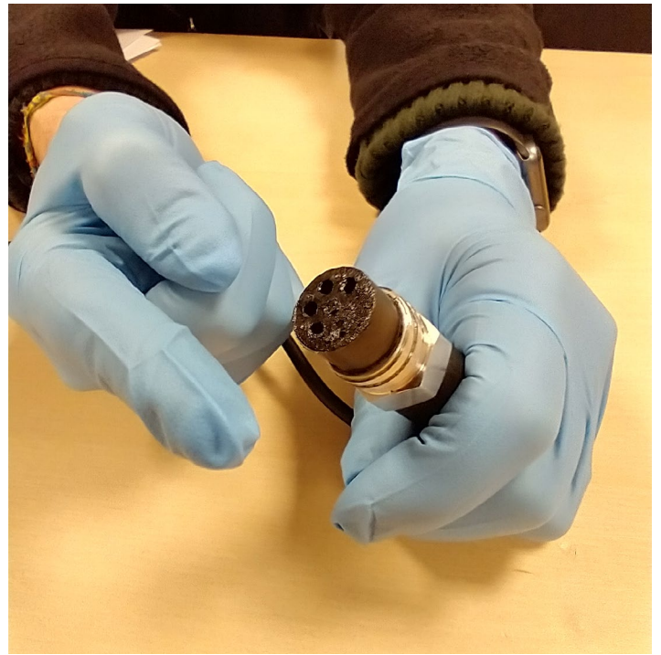
Figure 21: The connector plug with Molikote 111 applied
