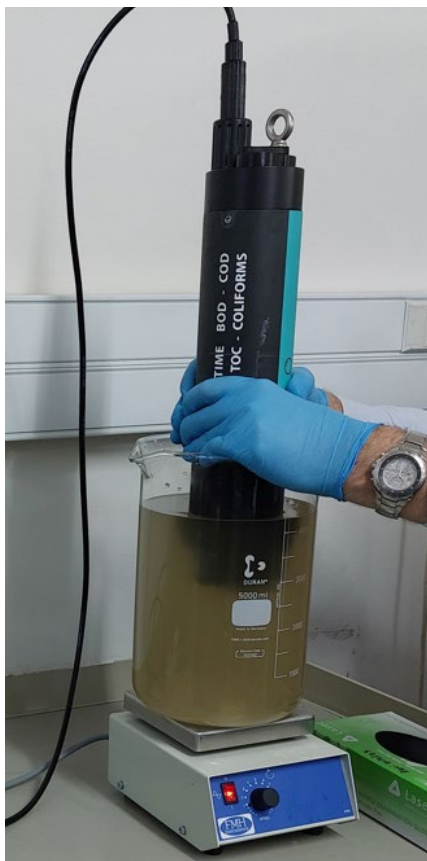
Figure 47. Example of spike test set-up in the lab. A vertical clamp is recommended for ease of measurement.
