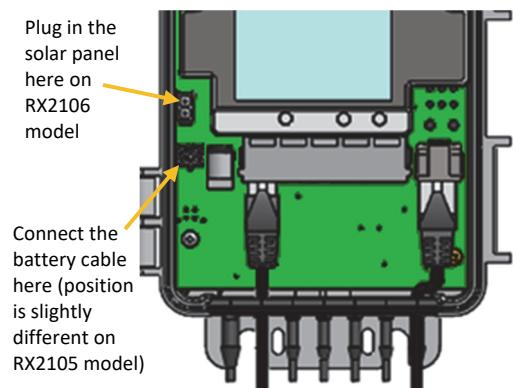
Once the battery cable is plugged in, "Initializing System" will flash on the LCD. A checkmark appears next to "System" after the station initialization is complete.
