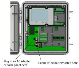
c. Once the battery cable is plugged in, "Initializing System" will flash on the LCD. A checkmark appears next to "System" after the station initialization is complete.
