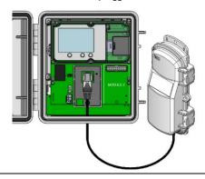
WARNING: If you inadvertently install modules while the power is on, you must disconnect and then reconnect the battery and charging device to guarantee proper operation.
