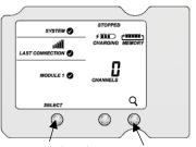
Press the Select button to switch to the module with RXW Manager installed
