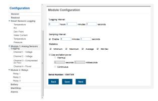
c. Click the Enable checkbox under Sampling Interval if you want to log statistics. Enter the sampling interval to be used for calculating the statistics (must be a factor of the logging interval). Select the statistics to be logged: minimum, maximum, average, and standard deviation. The selected statistics will be calculated between each logging interval at the sampling interval rate you select. Each statistical value will then be logged at each logging interval.
