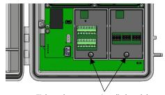
Tighten the screw on installed modules
