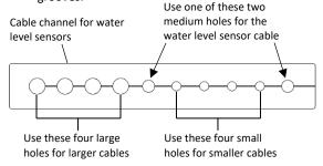
Important: The cable diameter must be 4.0 mm (0.156 in.) to fit through one of the smaller holes or 6.4 mm (0.25 in.) to fit through one of the larger holes in the rubber cable channel. If the cable diameter is too small, build up the diameter using heat shrink. If the cable is too big, splice on another cable with a smaller diameter to fit through the hole. If you are using the rubber cable channel designed for the water level sensor, reserve the medium holes for the water level sensor cable.
