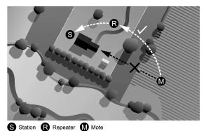
There should not be more than five motes in any direction at their maximum transmission range from the RXW Manager. Data logged by a wireless sensor must travel or "hop" across the wireless network from one mote to the next until it ultimately reaches the RXW Manager at the
