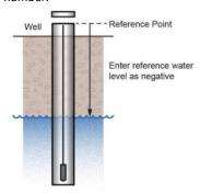
If the water level surface is above the reference point as shown below, enter the reference water level as a positive number.
