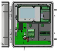
Plug in an Ethernet cable here
