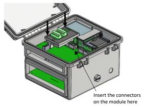
Tip: Install the analog module, water level sensor, or RXW Manager module on the left and the relay module on the right for easier cable routing.
