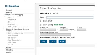
**Important:** Do not configure the water level and water flow channels yet. Configure any other sensors or relays as necessary, continue to step 11 to start logging, and then obtain a water reference level reading in step 12.
