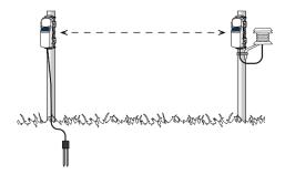
Make sure each sensor mote and repeater is positioned so that the built-in solar panel receives optimal sunlight throughout each season as shown. It may be necessary to periodically adjust the mote position as the path of the sunlight changes throughout the year or if tree and leaf growth alters the amount of sunlight reaching the solar panel.
