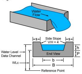
The HOBOlink water flow calculations for a trapezoidal weir assume the following:
