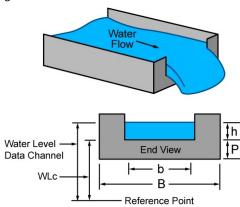
The HOBOlink water flow calculations for a rectangular weir assume the following:
