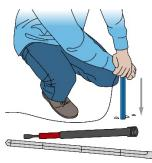
8. Once the probe is fully inserted in the hole, pack the soil around the top of the sensor to prevent water from
