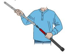
4. At the location where you want to install the probe, use a repetitive up-then-down motion on the slide hammer to vertically drive the pilot rod into the soil. Be sure to hold the slide hammer vertically without side-to-side movement. Drive the pilot rod in until it reaches the tape marking made in step 2.
