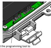
Connect the programming tool to these connection pins
