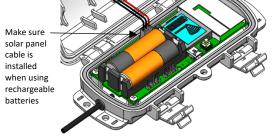
The mote contacts the network once the new batteries are installed. The green LED blinks quickly while the mote searches for a network to join and then blinks slowly while it completes the network registration. Once the mote has finished joining the network, the green LED turns off and the blue LED then blinks indefinitely while the mote is part of the network.
