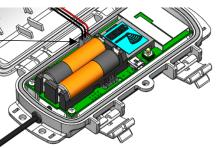
The mote contacts the network once the new batteries are installed. The green LED blinks during this process while the bars in the signal strength indicator on the LCD cycle from left to right and then the x icon blinks. Once this process is complete, the x icon is removed, the green LED stops blinking, and the blue LED begins blinking instead.
