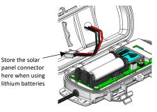
The mote contacts the network once the new batteries are installed. The green LED blinks quickly while the mote searches for a network to join and then blinks slowly while it completes the network registration. Once the mote has finished joining the network, the green LED turns off and the blue LED then blinks indefinitely while the mote is part of the network.
