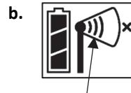
Once a network is found, the icon will stop flashing and the bars will cycle from left to right.
