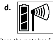
Once the mote has finished joining the network, the "x" icon is removed and the channel count on the station LCD increases by three (two for temperature/RH and one for the mote battery).
