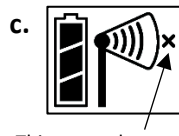
This network connection "x" icon blinks while the mote completes the registration process, which may take up to five minutes.
