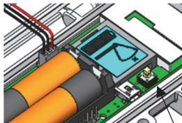
Open the door and install the rechargeable batteries. Press this button on the mote for 3 seconds.
