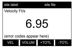
The default power up screen is already in BIG mode. If a different display mode is active, access the *Display Menu* by pressing the [DISP] key.
