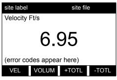
Use the [F1]-[F4],  $[\leftarrow]$  and  $[\rightarrow]$  keys to select the desired display parameter option. See Table 13 below for a complete description of the available options.
