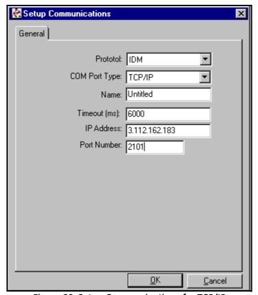
Figure 20: Setup Communications for TCP/IP
