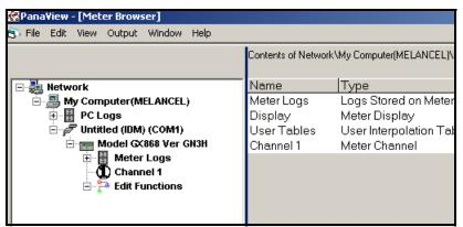
Figure 35: New Meter Browser with Meter Branch
