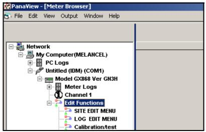
Figure 36: Meter Tree with Edit Functions Option
