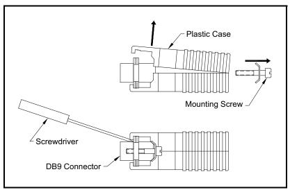
Figure 10: Opening the Converter Case
