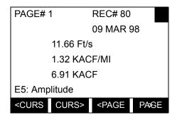
Use the  $[\leftarrow]$ ,  $[\rightarrow]$  and [F1]-[F4] keys to view additional records or to exit the log display. The options are listed in Table 15 below.
