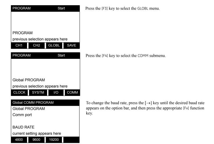
The available rates are 300, 600, 1200, 2400, 4800, 9600 and 19200 baud. After verifying or changing the baud rate setting, press the [EXIT] key three times to return to standard measurement mode.
