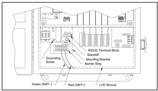
**Figure 9: Interface Converter Mounting**
