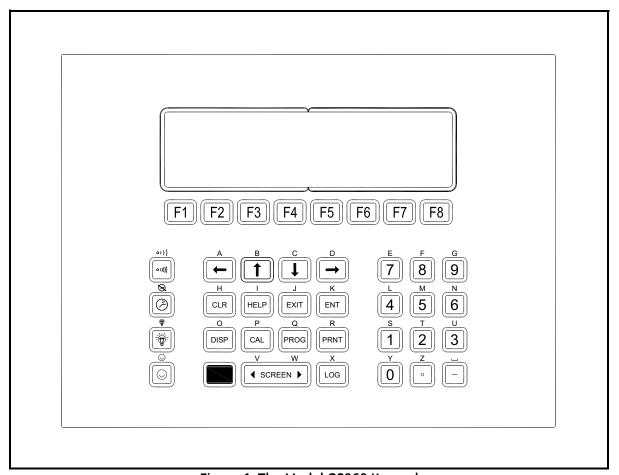
Figure 1: The Model GS868 Keypad
