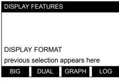
Press [F1] to select the BIG option. The measurement mode screen reappears with the display in the BIG format.
