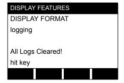
There are no log files currently stored in memory. Either all of the log files have been cleared or no log files have yet been created. Press any key to return to measurement mode.
