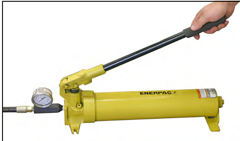
Figure 82: Pressurizing the Hydraulic Pump
