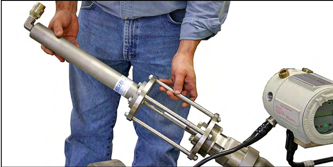
Figure 80: Installing the Insertion Mechanism
