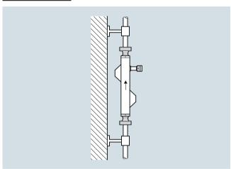
Vertical installation self-draining (upward flow)
