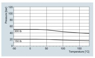
ASME-Flanges stainless steel AISI 326Ti/1.4571 to DN 100 (4")
