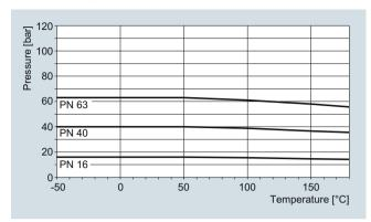
DIN-Flanges stainless steel AISI 316Ti/1.4571 to DN 100 (4")
