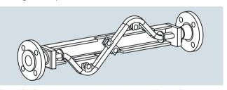
The MC2 Ex version sensor is based on a different Ex concept than MASS 6000. Therefore the MC2 Ex version sensor can only be connected to MASS 6000 IP67, MASS 6000 19" or SIFLOW FC070 standard versions, which have to be remote mounted in the safe area. MASS 6000 Ex d, MASS 6000 19" Ex and SIFLOW FC070 Ex can **not** be used with MC2 Ex sensors.
