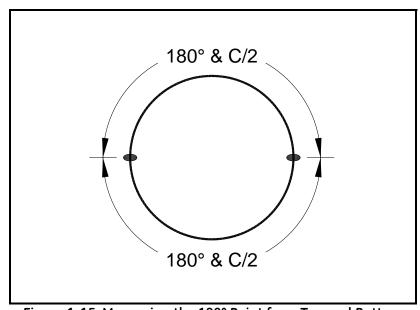
Figure 1-15: Measuring the 180° Point from Top and Bottom
