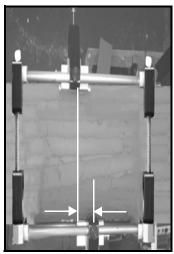
Figure 1-26: Distance Between Transducer Noses
