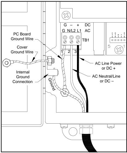
Figure 1-35: Wiring the Line Power
