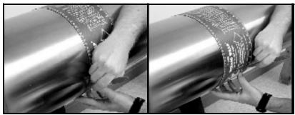
Figure 1-12: Marking Circumferential Lines on the Pipe
