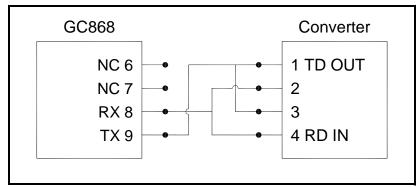
Figure 1-36: Typical RS485 Connections
