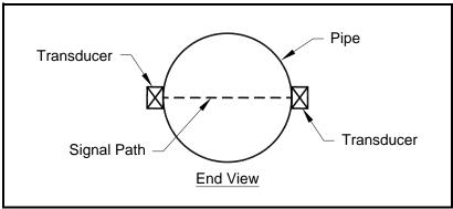
Figure 1-2: Desired Projection of Acoustical Signal Path
