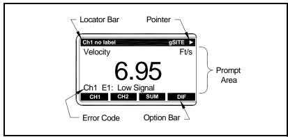
Figure 3-2: Display Screen Components
