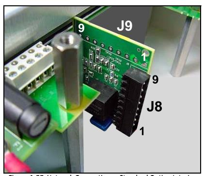
Figure 1-37: Network Connections - Standard Option Interior
