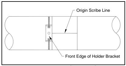
Figure 1-16: Lining up the First Bracket
