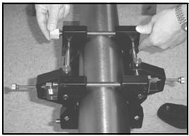
Figure 1-8: Installing Nuts onto the Fixture
