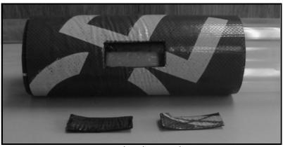
Figure 1-24: DMP-1 Material with Transducer Footprint Cut Out
