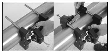
Figure 1-6: Mounting the Two Halves of the Fixture
