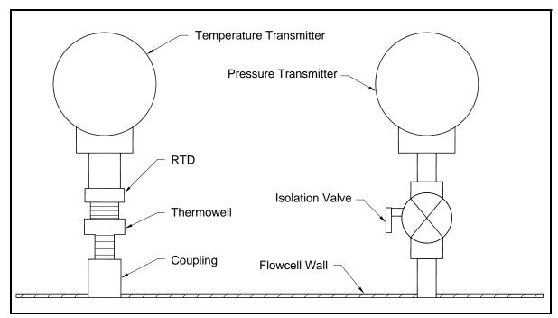
Figure 1-34: Typical Temperature/Pressure Transmitter Mounting
