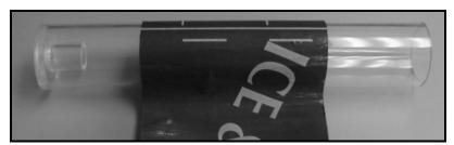
Figure 1-22: DMP-1 Damping Material Wrapped Around Pipe
