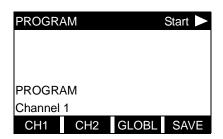
Press [F1] or [F2] to select the submenu for Channel 1 or Channel 2, respectively, from the option bar.
