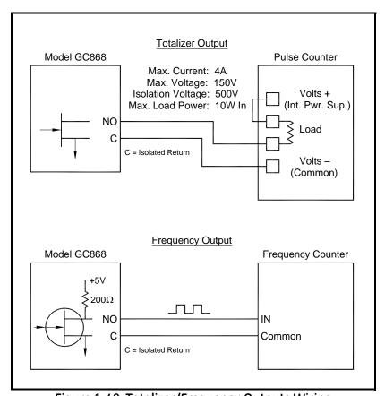
Figure 1-40: Totalizer/Frequency Outputs Wiring
