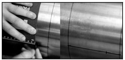
Figure 1-18: Measuring and Marking Spacing
