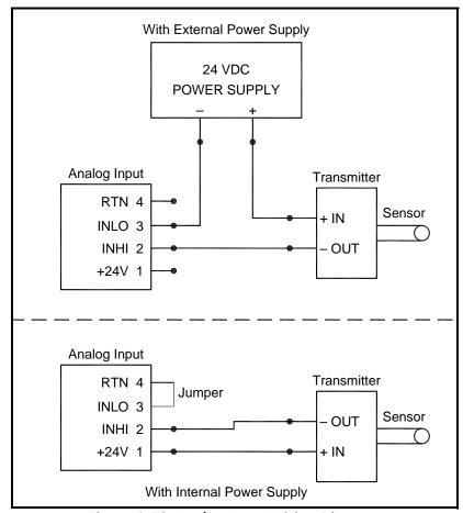
Figure 1-39: Analog Input Wiring Diagram
