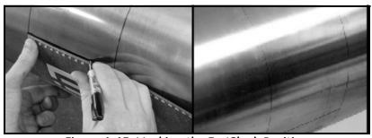
Figure 1-13: Marking the 3 o'Clock Position
