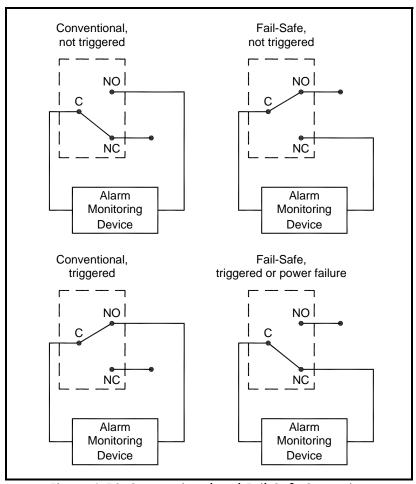
Figure 1-38: Conventional and Fail-Safe Operation
