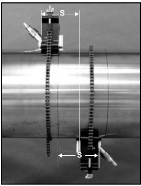
Figure 1-20: CFG-PI Fixture with Calculated Spacing
