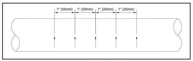
Figure 1-3: Measuring Thickness Along the Pipe Axis
