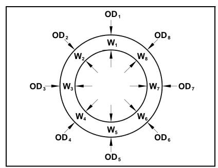
Figure 1-5: Measuring the OD and Pipe Wall Thickness
