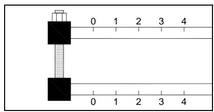
Figure 1-7: Fixture with Scale Origins Properly Aligned
