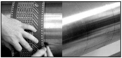
Figure 1-14: Marking the 9 o'Clock Position
