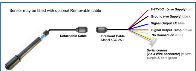
EC250 provides two calibrated analogue outputs (4-20mA) for EC and temperature over the Sensor Full Scale Range.
