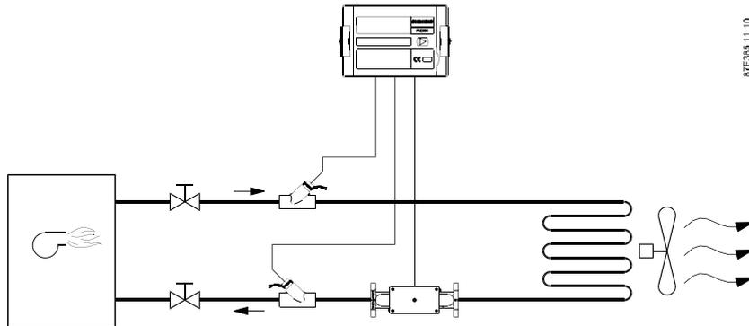
Figure 3-1 District heating applications with the flowmeter in the cold pipe
