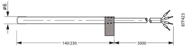
Figure 10-3 Pt500 temperature sensor, dimensions in mm (in)
