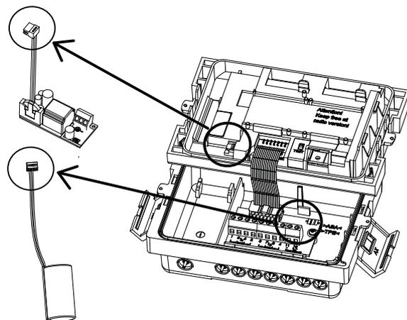
If the power supply module is not installed from factory, mount it as described below.
