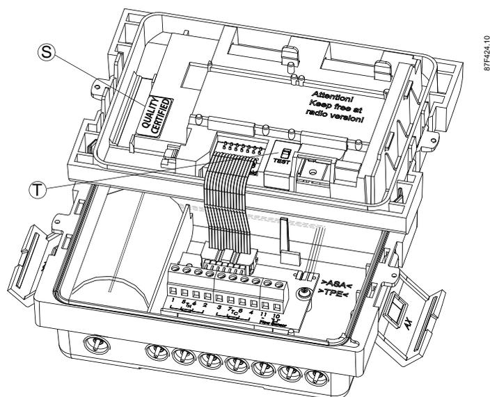
Figure 7-1 S - Verification sealing (protective seal); T - Test
