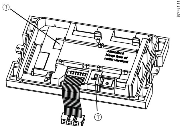
Figure 7-3 ① - Test output; T - Verification sealing / HW key
