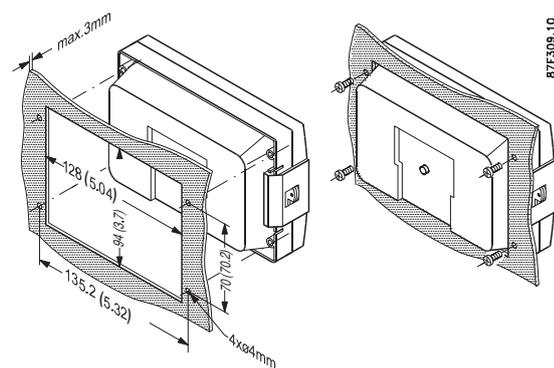
Figure 10-2 Panel mounting, dimensions in mm (in)
