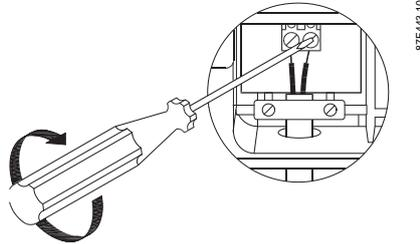
5. After installing main power cable, install protection cover using the two screws in order to avoid contact between voltage-carrying parts and cable-pull-relief, see figure below.
