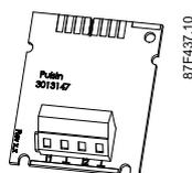
Figure 5-7 Pulse input module
