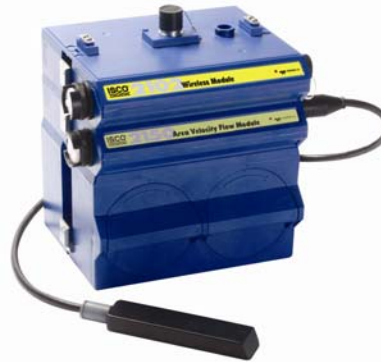
The 2102 wireless module stacks with 2100 Series flow modules and 2191 Battery Modules to provide a compact, integrated system for collecting and retrieving sewer flow data without repeated manhole entry.
